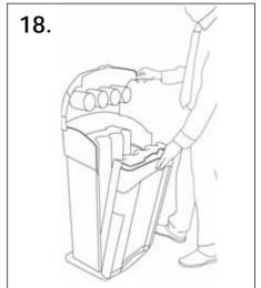
Tilt the door forward until the door is held in the open position.
