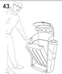
The stacking tubes can now be pivoted forward to reveal the fixing points for the sign.
