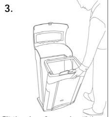
Tilt the door forward until the door is held in the open position.
