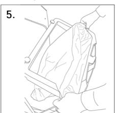
Install the correct size sack (406 x 727 x 1093mm-available from Glasdon) by firstly hooking onto the retention lugs at the front of the door.
