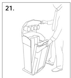
The door is now pivoted back clamping the sack between the stacking tubes.
