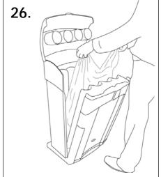
Tilt the door forward until the door is held in the open position and remove the sack.
