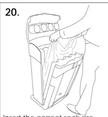
Insert the correct sack size (800mm x 1000mm- available from Glasdon) by lowering between the two halves of the stacking tubes.
