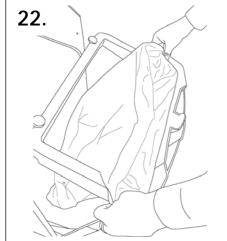
Once the door is in the closed position, secure the sack with the use of the sack retention clips.
