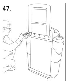
From the rear of the unit re attach the tubes using the screws removed in step 42.
