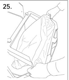
Remove the sack from the sack retention clips at the front and rear.
