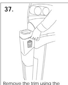
Remove the trim using the finger grip located at the front.
