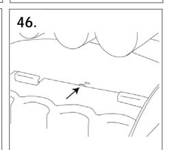
Now the sign is attached to the unit the stacking tubes must be re attached. Locate the tab on the stacking tubes with the main unit.
