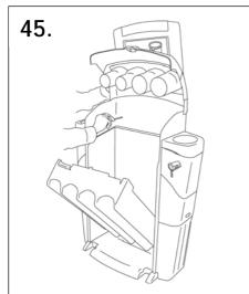
Using the 5 screws provided screw the sign to the unit as shown.
