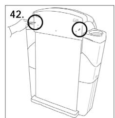
From the rear of the bin remove the upper two stacking tube fixing screws using a screwdriver (keep the screws to hand).
