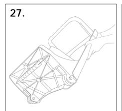
Two casters are located at the front of the door which allow it to be tilted and wheeled from the body providing excellent access.
